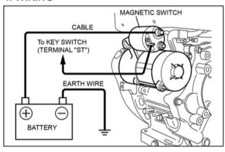
(1) Connect positive (+) terminal of the magnetic switch and positive (+) terminal of the battery with battery cable.
